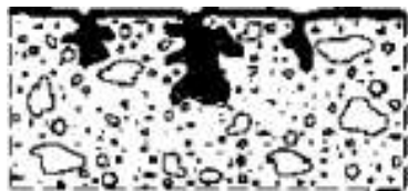
Picture depicted Nippon Densifier L applies on surface, penetrates and seals the pore with hard crystalline form
